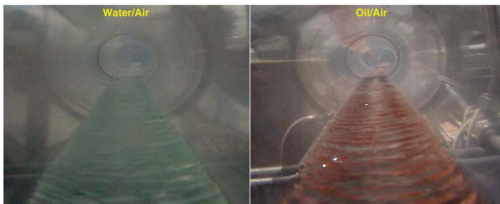
Fig. 12—Stratified wavy flow pattern with 3D wave structure for water/air and oil/air flow.
