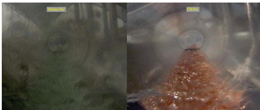
Fig. 14—Stratified wavy flow onset of atomization for water/air and oil/air flow.
