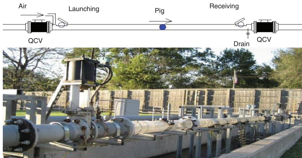
Fig. 3—Picture of QCVs and schematic of pigging system.
